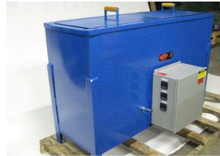
Typical Model of rectangular tank is shown herewith. Inside dimensions; 24" x 24" x 18". Capacity; 44 gal. Temperature range 250° to 550° F. 480-V, 3 phase 60 cycle.
