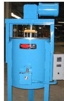
Model 25GMB, 25 gal. motor agitated glue tank
